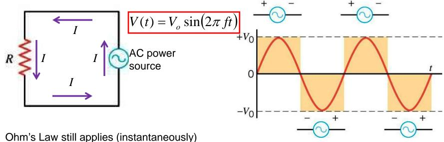
$$I(t) = \frac{V(t)}{R} = \frac{V_o}{R} \sin(2\pi ft) = I_o \sin(2\pi ft) \iff \text{The sine function can give both a positive or a negative value, depending on the argument}$$
