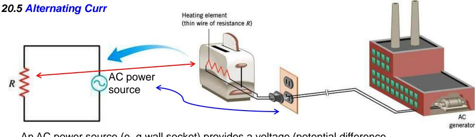
An AC power source (e..g wall socket) provides a voltage (potential difference between the two terminals) that reverses direction periodically. The resulting current in the circuit also alternates direction with the same frequency.
