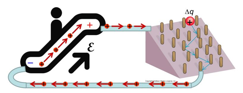
$$P = \frac{\Delta W}{\Delta t} = \frac{\left(\Delta q\right)V}{\Delta t} = \frac{\Delta q}{\Delta t}V = IV$$
