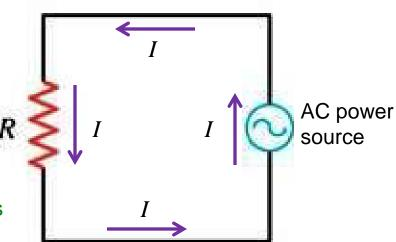
Because they allow us to use the same equations as DC, we use rms values for voltage and current when specifying AC circuits. Also: the *rms values for voltage* and current are the DC values that would deliver the same power
